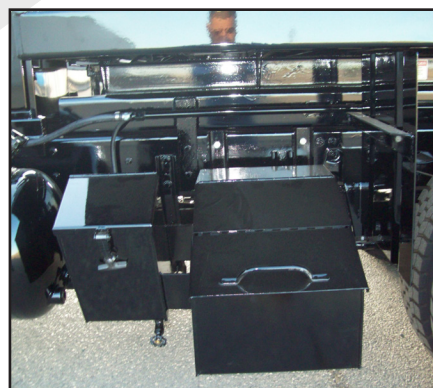
Sand box carries base material for deeper potholes and a solvent dip tank to clean tools before and after patching.
