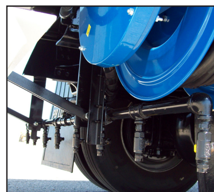
Spray bars allow your pothole patcher to double as a liquid asphalt distributor when necessary.
